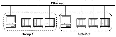
To reduce the amount of network traffic on a public use Ethernet network, the PC and the measuring stations can be connected via their own independent network. In this case, the PC and the measuring stations should be in the same IP subnet. For example, as shown in the following figure, each PC has two Ethernet NICs, one for connecting with other PCs and one dedicated for use with the WE7000 measuring stations. The two cards are configured with different IP addresses.
